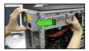
To install a power supply module:
